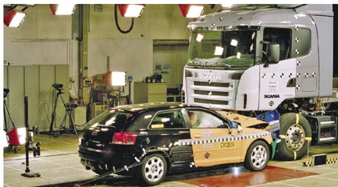
Truck collision Testing of Front Underrun Protection
